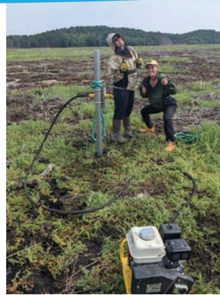
Katie (left) and Molly use a vibracore, courtesy of Northeastern University's Marine Science Center. The vibracore uses a generator and a repurposed concrete mixer to vibrate an aluminum tube into the ground, allowing them to retrieve more than six feet of relatively undisturbed sediment and bring it back to the lab for analysis.
