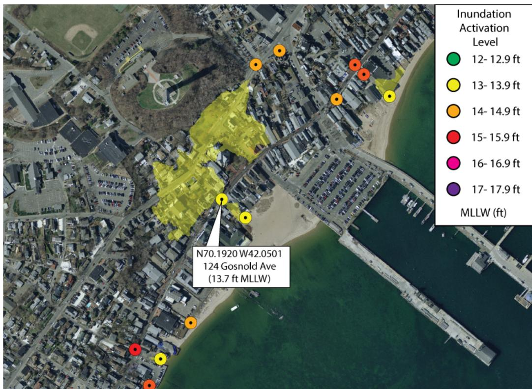
Figure 9. Example of colored coded inundation pathways that match the tide staff elevations in MLLW ft.
