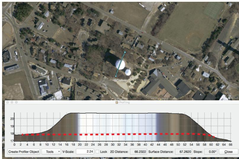
Figure 5. Example of ‘pull up’ near water tower in Provincetown. Dotted line is more representative of elevations at the water tower. Blue line in image is location in profile. Profile units = meters (Vert. NAVD88, Hor. NAD83).
