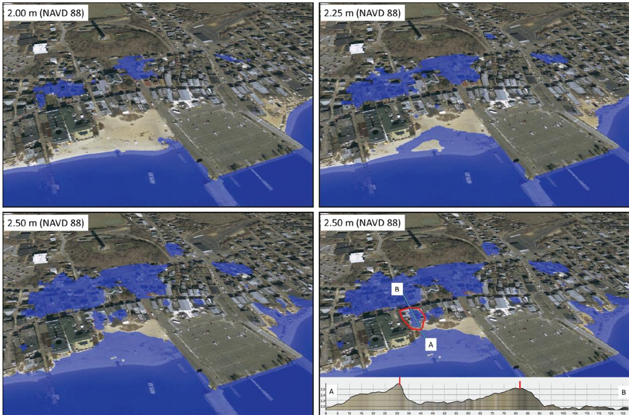
Figure 4. Downtown Provincetown, draped aerial photograph over Lidar surface. Blue areas are horizontal plane created in Fledermaus at increasing elevation. Lower left is example of a storm-tide pathway with accompanying profile. These images were generated before field work to identify potential IPs.
