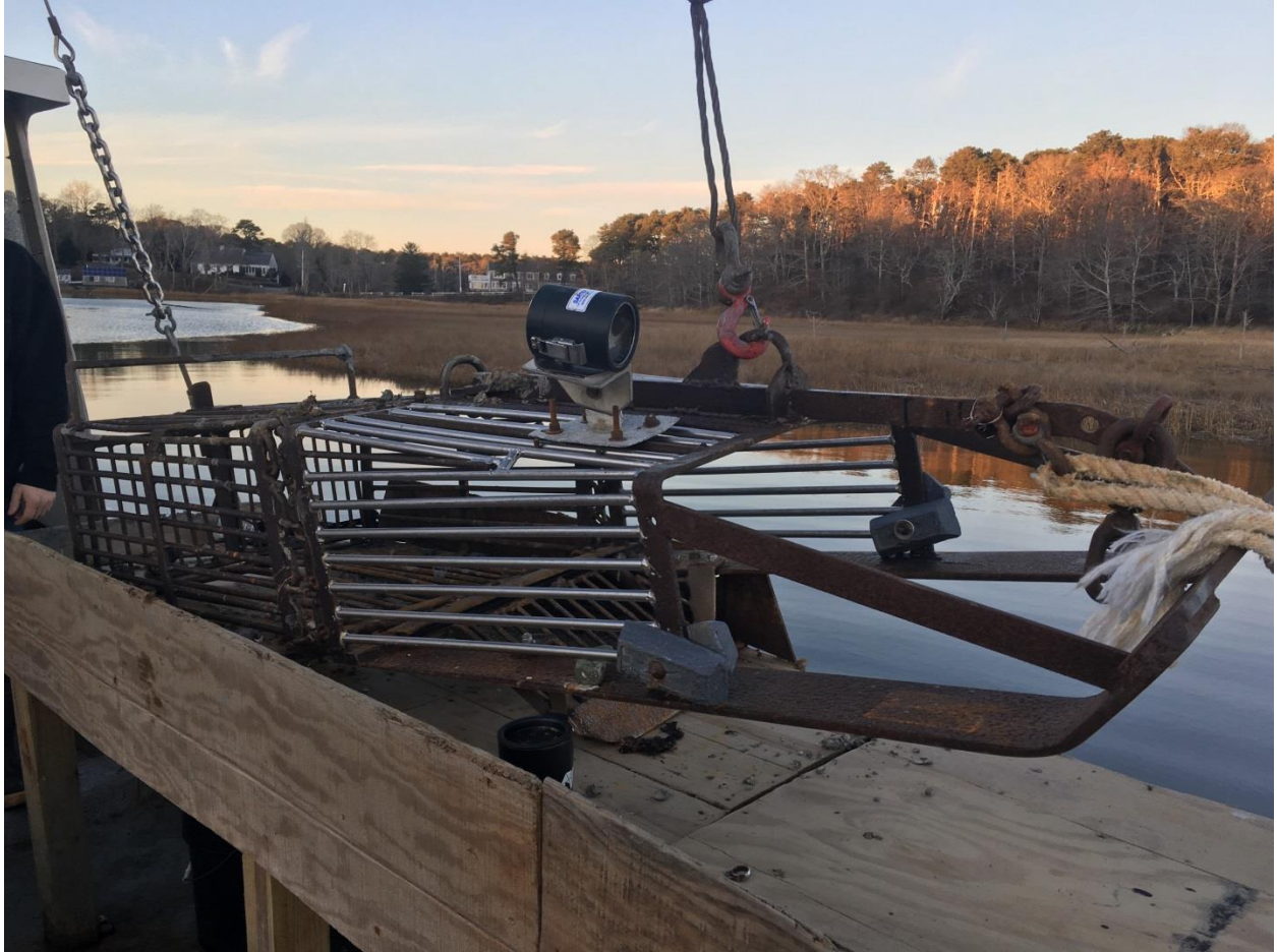
Figure 3. Dredge used for quahog surveys. Note camera housing mounted on top of dredge frame.
