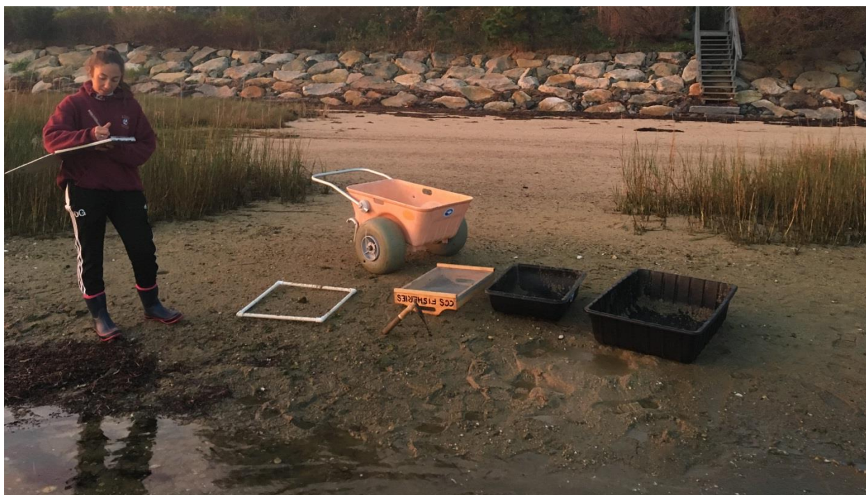
Figure 4. Intertidal shellfish sampling. Left to right: 0.25 m 2 quadrat, 6 mm screen and clam rake, basins.
